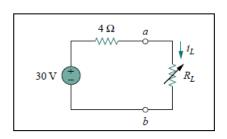
When  $R_L = 6\Omega$ ,  $i_L = \frac{30}{4+6} = 3$  A. When  $R_L = 6\Omega$ ,  $i_L = \frac{30}{4+16} = 1.5$ A and when  $R_L = 36\Omega$ ,  $i_L = \frac{30}{4+36} = 0.75$ A **2. Find the Thevenin equivalent of the circuit in figure.**
