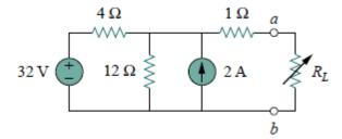
**Ans.** We find  $R_{Th}$  by turning off the 32-V voltage source (replacing it with a short circuit) and the 2-A current source (replacing it with an open circuit). The circuit becomes what is shown in figure (a).
