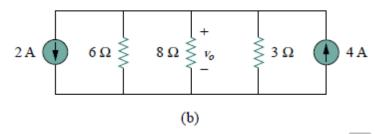
We also combine the 2-A and 4-A current sources to get a 2-A source. Thus, by repeatedly applying source transformations, we obtain the circuit in figure (c).
