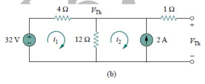
For loop (1),  $-32 + 4i_1 + 12(i_1-i_2) = 0$  and for loop (2),  $i_2 = -2$  A Solving for  $i_1$ , we get  $i_1 = 0.5$  A. Thus,  $V_{Th} = 12 (i_1 - i_2) = 12 \times (0.5 + 2) \text{ V} = 30 \text{ V}$
