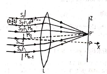
normally on N parallel slits. The light is diffracted through N slits and is focussed by a lens L on the screen Z placed in the focal plane of L. The wave diffracted from all the slits in direction  $\theta$  are equivalent to N parallel waves, each wave starting from midpoints,  $S_1, S_2, \ldots S_n$  of the slits.
