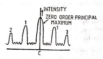
hofer diffraction pattern due to N parallel equidistant slits. The pattern consists of a central maximum called Zero order principal maximum followed by a number of principal maxima on either side. There are (N-1) equi-spaced minima between any two consecutive principal maxima.
