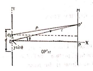
co-ordinate system with x as abscissa and y as ordinate. The slit is divided into a large number of infinitesimal elements of equal width dy. Consider one element dy at a distance y above the origin. Consider a point P' defined by a possible diffracted beam making an angle  $\theta$  with the normal to the plane of slit. Let OP' = r and the element dy is at a distance  $\rho$  from P'.
