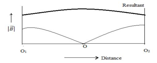
As evident from above graph, the resultant induction remains uniform over a finite region about the midpoint of the two coils. The total magnetic induction at a midpoint due to both the coil is
