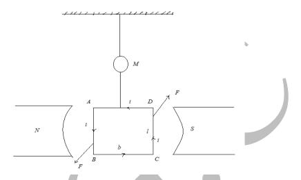
The ballistic galvanometer consists of a rectangular coil ABCD having n turns of wire wound on a non conducting frame. The coil is suspended by a suspension fibre in a uniform radial magnetic field of flux density  $\vec{B}$  provided by a permanent magnet whose pole pieces are N and S. The suspension fibre has a small mirror M. The deflection of the coil can be measured by the usual lamp and scale arrangement.
